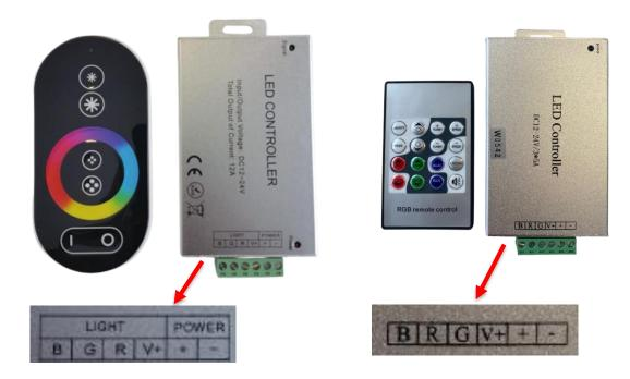
The new RGB controller is fully backwards compatible for the affected coffee machine series under considering that the cable strands are plugged in correctly. New order is blue, **green**, **red** compared to the old it is blue, **red**, **green**. Existing spare parts on stock (old version) can be still used.
